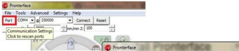
7) Now press the **Connect** button. The program will try to connect to the machine.
