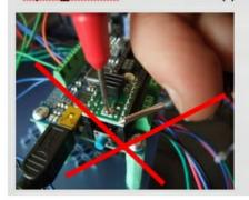
With smoothieboard, no need use screwdriver and turn potentiometer to setting with difficulty the limit of current, like drivers of a lot of 3d printer.
